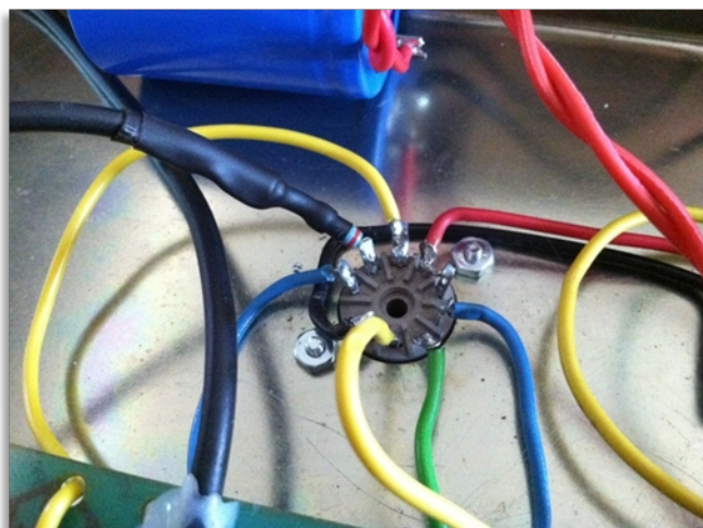
V1 socket and hot-shield cable – photo C.
