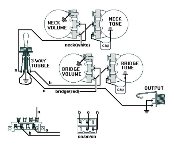
Solder red and green wires on neck pickup and tape connection. Solder black and white wires on bridge pickup and tape connection.
