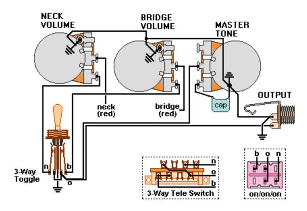
For each pickup, solder the black&white wires together and tape up each connection. The green&bare wire of both pickups go to ground.
