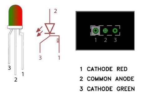
The diagram above shows the pin-out, schematic symbol and pad connection for a common anode LED.
