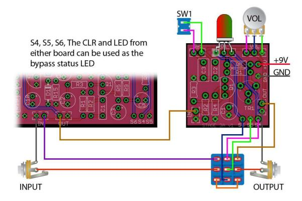
Note: you can use the bypass status circuitry (S4, S5, S6, CLR & LED) from either board.
