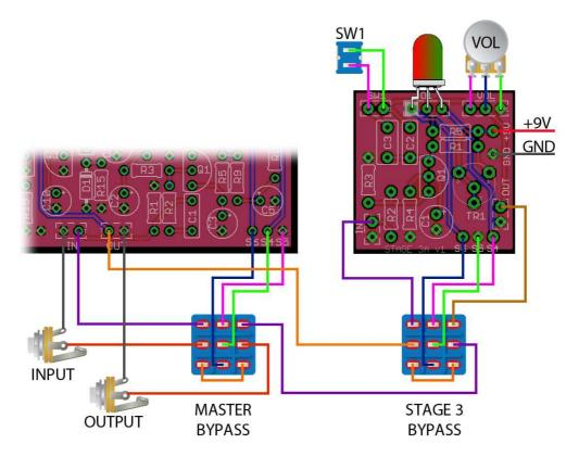
The bypass status circuitry (S4, S5, S6, CLR & LED) from the first board is used for the standard bypass status indication and obviously the bypass status circuitry on the Stage 3A board is used for Stage 3 bypass status indication.
