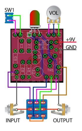
When using the Stage 3A in tandem with another circuit it is possible to switch the Stage 3A in and out of the circuit by using two 3PDT footswitches. The first footswitch (Master Bypass) works like a standard bypass switch, switching both circuits in and out; the second footswitch is used to switch the Stage 3A.
