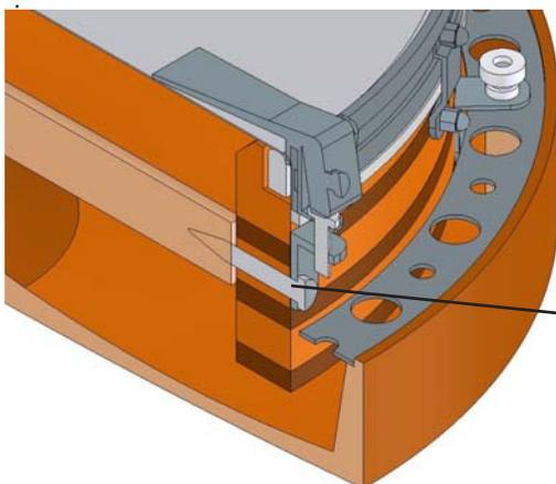
Tailpiece bracket and mounting assembly. Since the hole through rim was oversized to allow the drill extension, you may need to shim the screw that goes into the dowel stick
