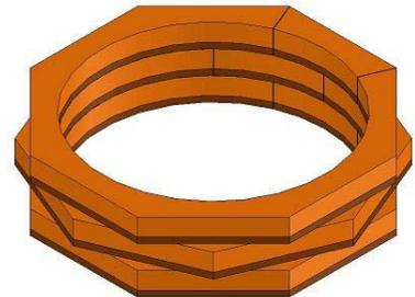
The next step is to sand and shape the rim. A lathe could be used for this step, but was easy enough to use the disk and drum sanders. A step then needs to be cut in the top of the rim to allow the tone ring to sit. A groove 1/2" deep by 3/8" wide was cut using a straight router bit and router table.
