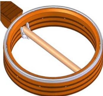
T-nut with sides cut and fitted into the holes previously drilled into the rim. The set screws adjusted from the bottom will push the tone ring upward against the head.
