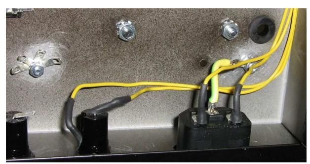
Before assembling the yellow wires please connect the power cord and check with your multimeter, that it will show 0 Ohm between chassis and earth (I always measure against earth in the wall outlet to be absolutely sure) and 0 Ohm between the star ground lug and earth. Please disconnect the power cord before going on wiring the power supply!
