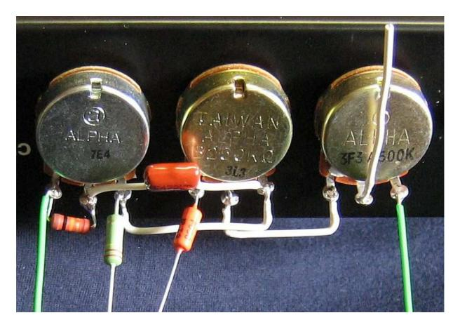
Last assemble the controls to the chassis, connect the wires and do the connections to the channel switch for channel 1 (see picture).
