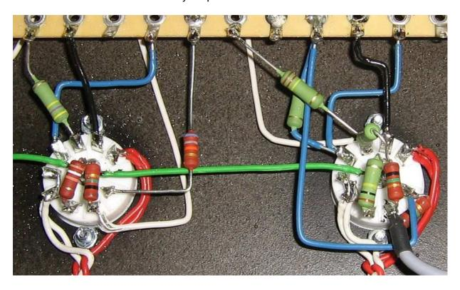
Next do the remaining wiring for the channel switch as shown in the layout plan. Then do the wiring for the gain control (VR4), to ease up the assembly attach the variable resistor to the front panel the wrong way round and wire it before putting it into the chassis (see picture). The connecting wires attached to the controls only should have a length of 3cm (green) and 6cm (white) respectively, don't solder the center lug now.
