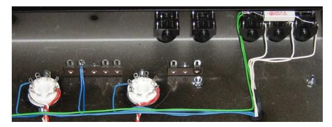
Then connect the secondary side of the output transformer to the output plug sockets (speaker outlet) with green and white wire and assemble the security resistor R57 (this resistor prevents the output transformer from damage, when no speaker is connected). Please connect all ground connectors of the three output plug sockets with a wire (see picture), then assemble R57 and connect the output transformer:
