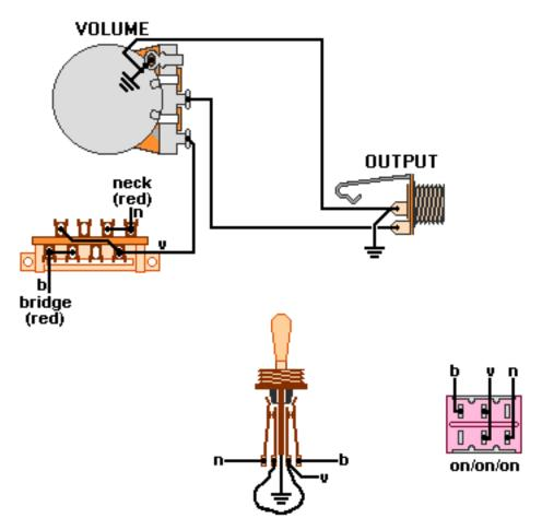
For each pickup, solder the black&white wires together and tape up this connection. The green and bare wires from both pickups go to ground.
