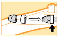
**Step 3** Add one of the metal spacers provided, and reinstall the adjusting nut. This truss rod is rescued and ready to work like new.
