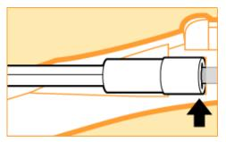
**Step 2** The threading die cuts clean threads on the newly exposed truss rod. Now the rod is ready for the adjusting nut again.
