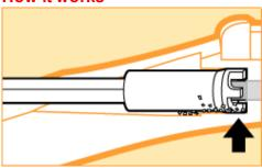
**Step 1** The cutter removes wood around the damaged rod, making room for new threads.
