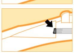
**The problem:** A truss rod nut that's become cross-threaded, frozen, or broken off competely. You can't adjust the neck, and the trouble is hidden below the surface.
