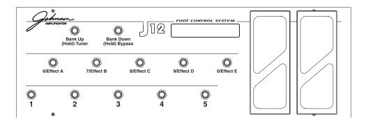
The front panel of the J-12 consists of a 20 character vacuum-fluorescent display, ten programmable footswitches, a dedicated bypass footswitch, a Select switch, and two built-in expression pedals.
