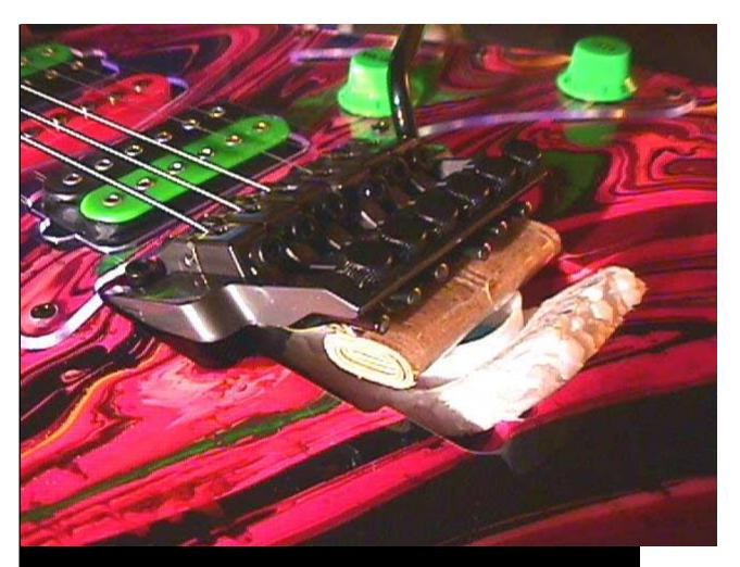
But if I'm just doing someting quick I'll more than likely grab my clamp. Throw the bar in the trem and clamp it to the body. Notice the cloth over the body to prevent dents or scuffs, and the styro wrap around the clamp shaft to prevent anything else. The red feet of the clamp accessorize this DNA well, and are rubber for soft grip and stick.
