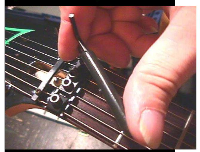
Time to put the truss rod cover on while I'm here. I'm going to adjust the pickup height now, a #1 flathead screwdriver will do. Turn the screw clockwise to raise the pickups, counterclockwise to lower. Set them where you like them just not so close the magnetic field affects the strings, this will kill sustain and sometimes pull the string slightly sharp. This is where I set mine.
