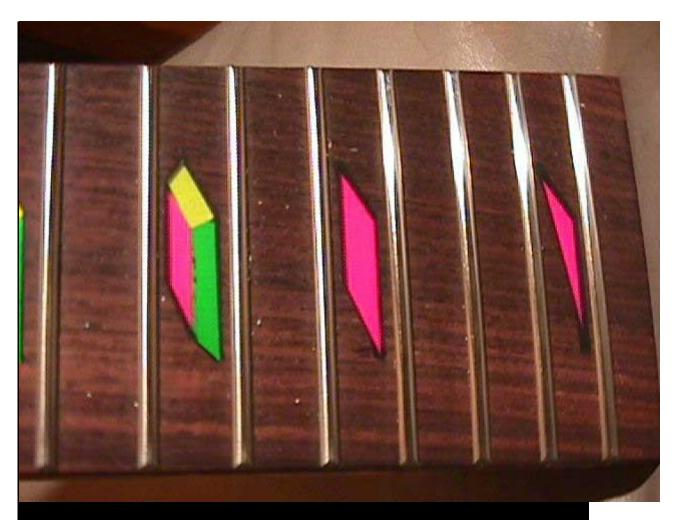
30 minites later the frets are shining. I'm cleaning the board of all the wool fibers and dust with an old toothbrush. It gets it out of the pores and from against the frets very well.
