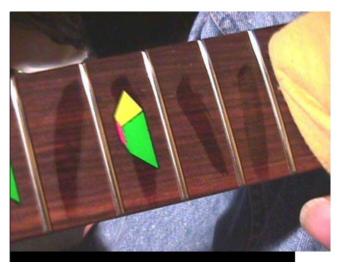
Go back and spread it around making sure to get right up against the frets. Reload and continue on till the board is covered. By the time you get to the end it's time to start buffing the excess off where you started. Buff till the wood is obviously no longer leaching oil.
