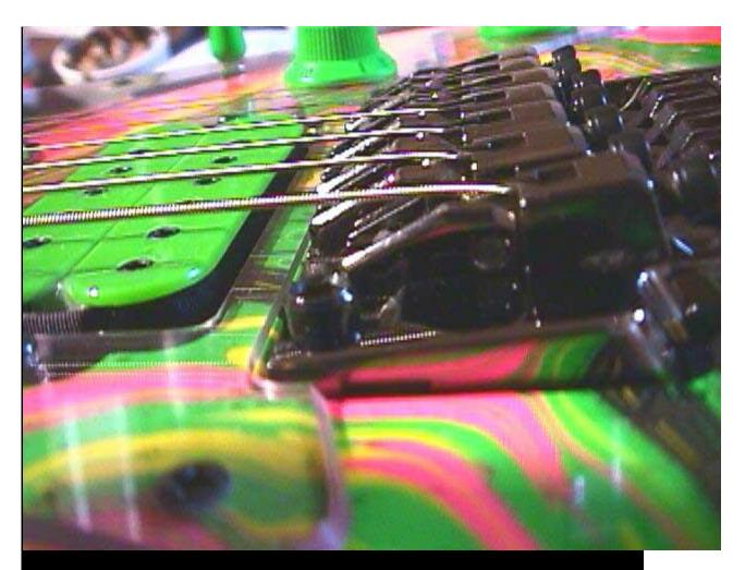
After the height is right it's time to check all the frets. Fret every note on the board to make sure you don't have anything choking on a high fret. On the unwounds do this by bending the string at least a full step to check for areas that choke. I like at least 3+ steps of clean tone and why I set my trebble side at 1.5mm. You might have to readjust the action slightly depending on the neck and how good your eve was at setting it up. :-)
