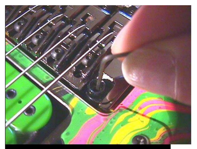
Here is a pic of the post with the set screw extended. They screw out the bottom and will not come out through the top of the post. The set screw locks the post threads against the threads of the post anchor and is critical to eliminate play between them, causing tuning instability.
