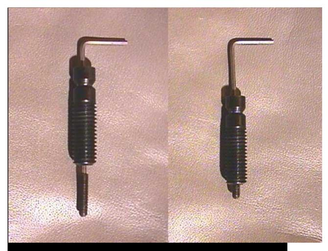
Now I can go ahead and adjust the action height using the 4mm allen wrench in the trem posts. If the trem posts bottom out and the action still isn't low enough, guaranteed more neck shim is needed. Go back to page 6 for details.
