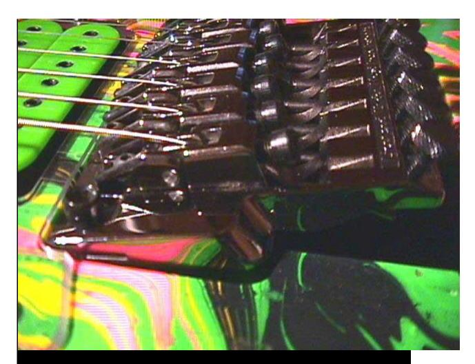
If you can't tell why you should vist the <u>Trem Angle</u> part of the Tech section. The trem is angled far forward and I'm not close to tune yet. One quick look inside the trem cavity tells me the claw is way too far out. Screw the claw in to add enough string tension for 009's. I'll eyeball this in to about where I know it should be.
