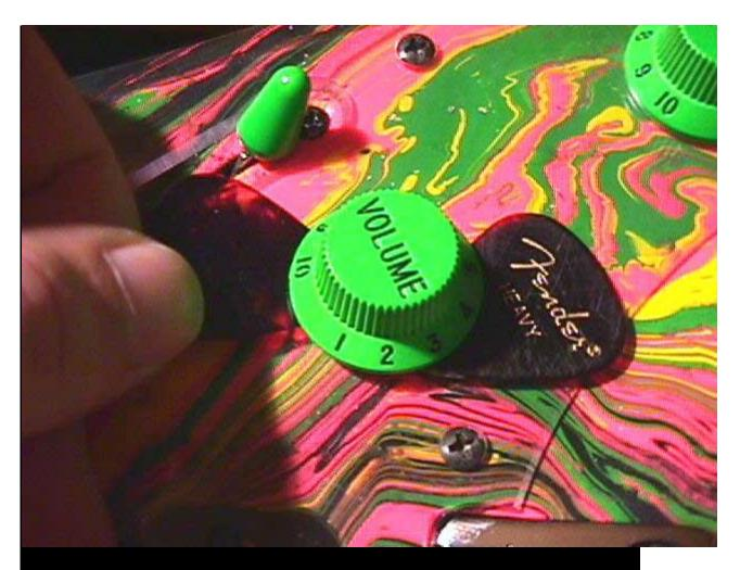
The switch tip will come off with your fingers if it's been off before. If it hasn't the chances are you'll need to use a pair of pliers. Use your rag to protect the plastic and only squeez hard enough to grip the tip. I'm using channel locks to get the right jaw opening, pinching more underneath the tip.
