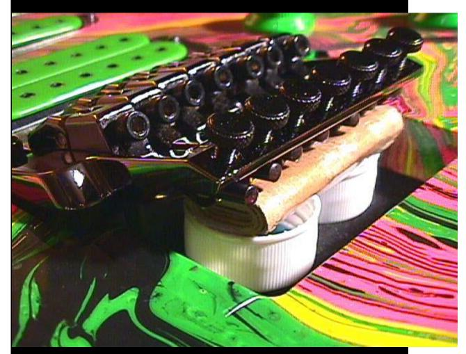
This is how I would block a Jem trem, notice the bottlecap wedged into the crushed styrofoam that's conformed to the claw.
