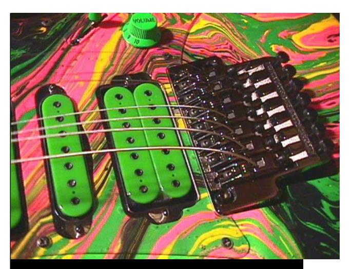
As good a time as any to adjust all the fine tuners to the same height. Make sure they're screwed in enough to have 2 full turns of adjustment to back out.
