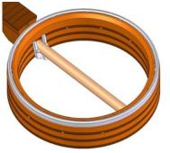
T-nut with sides cut and ~ fitted into the holes previously drilled into the rim. The set screws adjusted from the bottom will push the tone ring upward against the head.
