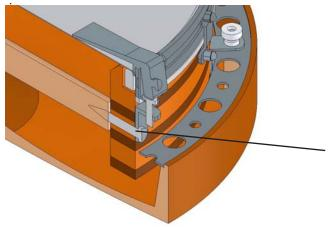
Tailpiece bracket and mounting assembly. Since the hole through rim was oversized to allow the drill extension, you may need to shim the screw that goes into the dowel stick
