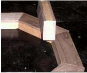
I also cut the inside rounded edge before gluing the small pieces together. This made it easier to sand and shape after the final assembly.
