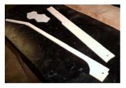
more than once, you may want to glue your paper patterns to some 1/4 plywood so your templates last. Trace the top and side views on your stock. Before cutting them on the band saw, you may want to cut the groove for your truss rod now. I liked the style of a 2-way truss rod called a Hot-Rod truss rod. It allows
