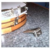
Once again, buying the components can make more sense than fabricating them. On the website, I have patterns available for the adjustable tailpiece. I had to go back a month after it was finished and reinforce the main joint with a piece of 1/8" thick brass bent in an "L" shape. The strings exert much more force on the structure than I originally expected. Two months later, the repair is still holding and I expect it to last.
