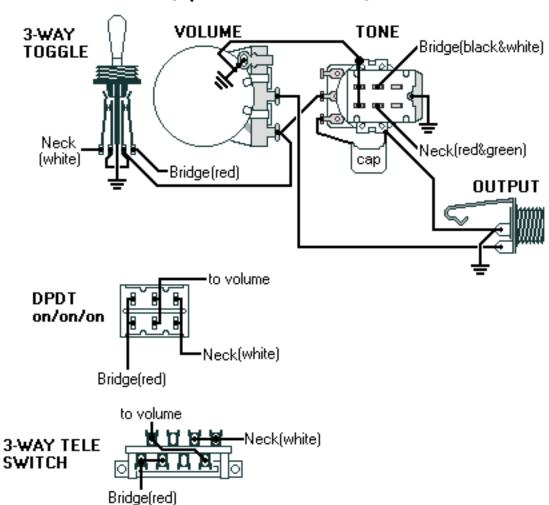
All other pickup wires not shown or mentioned go to ground. Note: Tailpiece should be connected to common ground. All grounds 🛓 must be connected.
